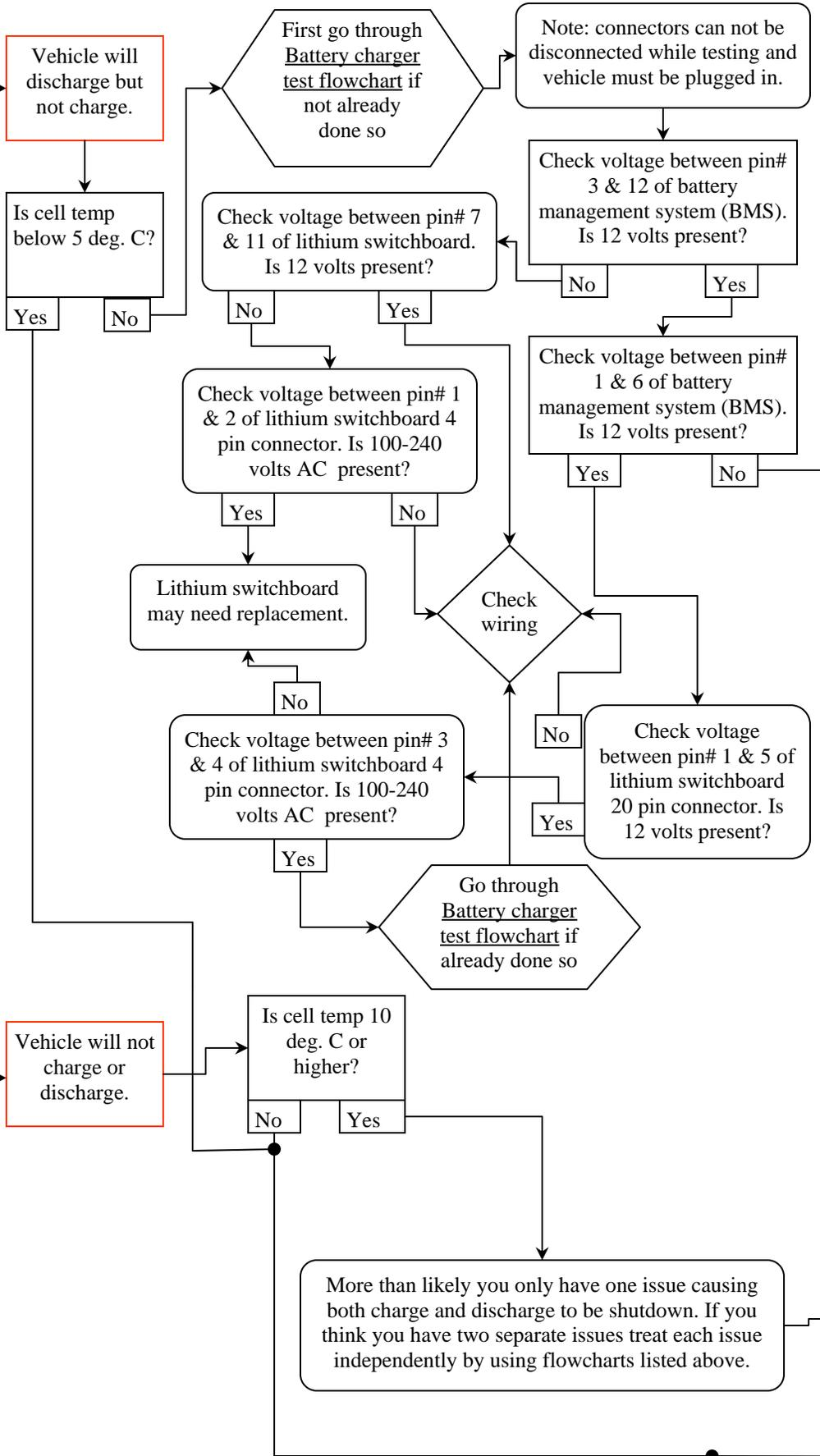
**Note that if any cell connections need to be disconnected/tightened/ repaired or modified in anyway the main battery disconnect must be turned off and the lower front 36 pin connector or the BMS must be disconnected! If not done the BMS has a extremely high chance of developing an internal issue.**
